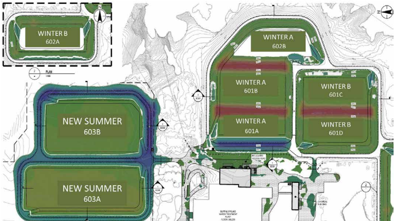
Figure 3: The layout of the new ponds as part of Plant Renewal. Total pond volume will be sufficiently increased to contain all wastewater inflows and eliminate the current practice of continuous overflow. When combined with substantial reductions of wastewater produced by the upgraded plant, the hydraulic and sludge overloading problems that plague the current lagoon system will be resolved. Non-compliances of environmental regulations for residual waste discharged to the environment will be a thing of the past. This will maintain a healthy watershed ecosystem and ensure source water protection for aquatic life and downstream users. NOTE: Refurbishment of Winter Pond B 602A was descoped from the project in 2025.
