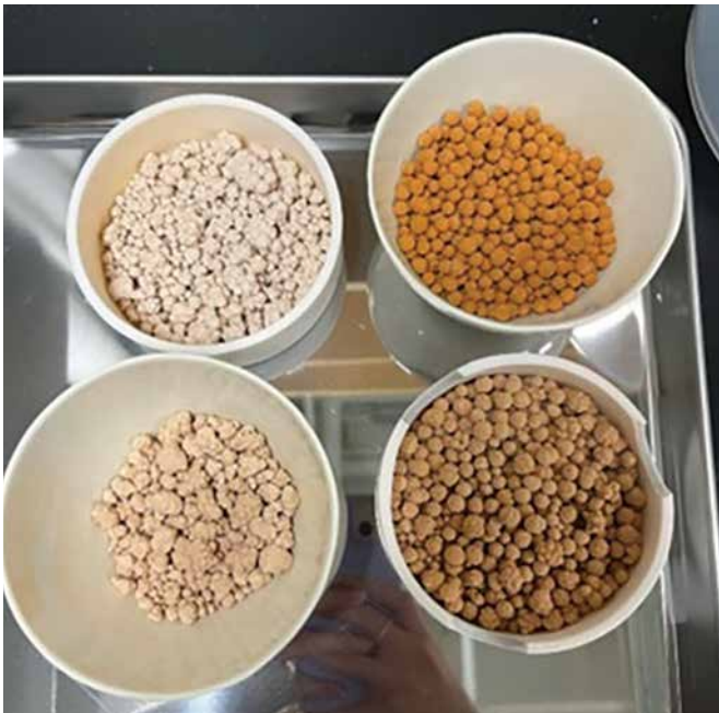
Figure 10: Ceramsite granules made with water treatment sludge and clay. (Credit: CSCE/SCGC Moncton 2023, paper # 8270.)
